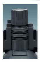
The Type 546 Ball Valve stem utilizes a predetermined break point opposite the media side of the stem seals. This break point is a groove with an inner diameter that is less than the stem seal grooves. This ensures that if there is a stem failure, the failure will occur at that point and media will not leak to the outside of the valve.
