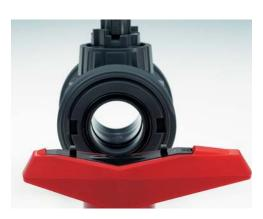
The Type 546 Ball Valve seat carrier is reverse threaded while the valve nut utilizes a standard thread. This ensures that the seat carrier is not inadvertently tightened when the valve nut is tightened and avoids possible stem failures.
