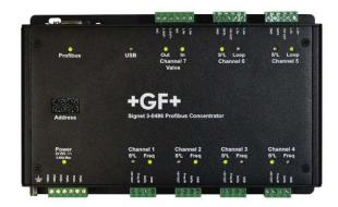
The Signet 0486 Profibus Concentrator allows for simplified connection of Signet sensors to a PROFIBUS network. The 0486 supports six sensor interfaces and a 4 to 20 mA current loop proportional valve interface. The 0486 supports PROFIBUS DPV1 and is available with either DB9 or M12 network connectors.
