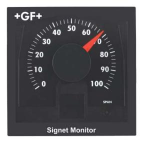
Sensor Powered - external power not required.
