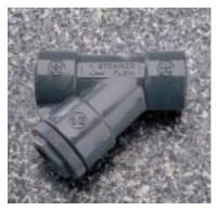
Strainers, with a 100 mesh screen, should be used to assure proper pump check valve performance when solids are present in the supply fluid. Allow for a 1 PSI maximum pressure loss through a clean screen.
