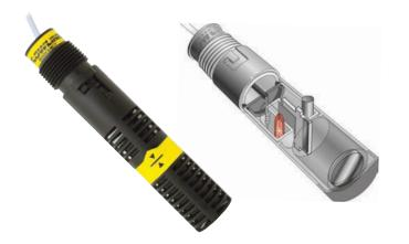
The general purpose buoyancy point level switch provides reliable liquid level detection of relatively clean water and chemical solutions with a 15VA reed switch output. Media examples include boric acid and ultrapure water. The baffle body eliminates level switch chatter caused by turbulence. The submersible polypropylene or PVDF liquid level sensor is mounted vertically inside the tank as a high level alarm or low level alarm.
