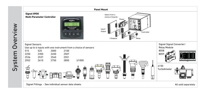
There are hundreds of system types that can be set up with the 8900. The examples below illustrate various sensors in different installation schemes. Wiring topology for point-to-point, daisy-chain, multi-drop, or a combination of these are listed in each example. Digital sensor outputs allow for long cable runs with high noise immunity. See Wiring section for allowable cable lengths.
